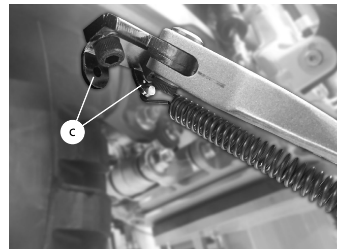
c) Adjustment holes in the side stand
