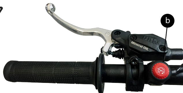
b) Stop button, to the left of the handlebar
