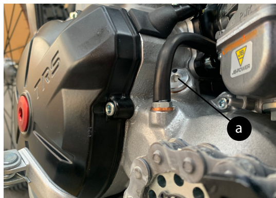
a) Oil filler cap, in the upper part of the sump.
