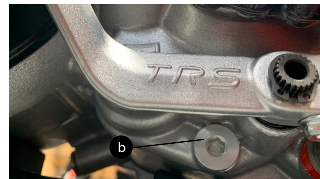
Fig (b): Oil drain plug at the bottom of the sump
